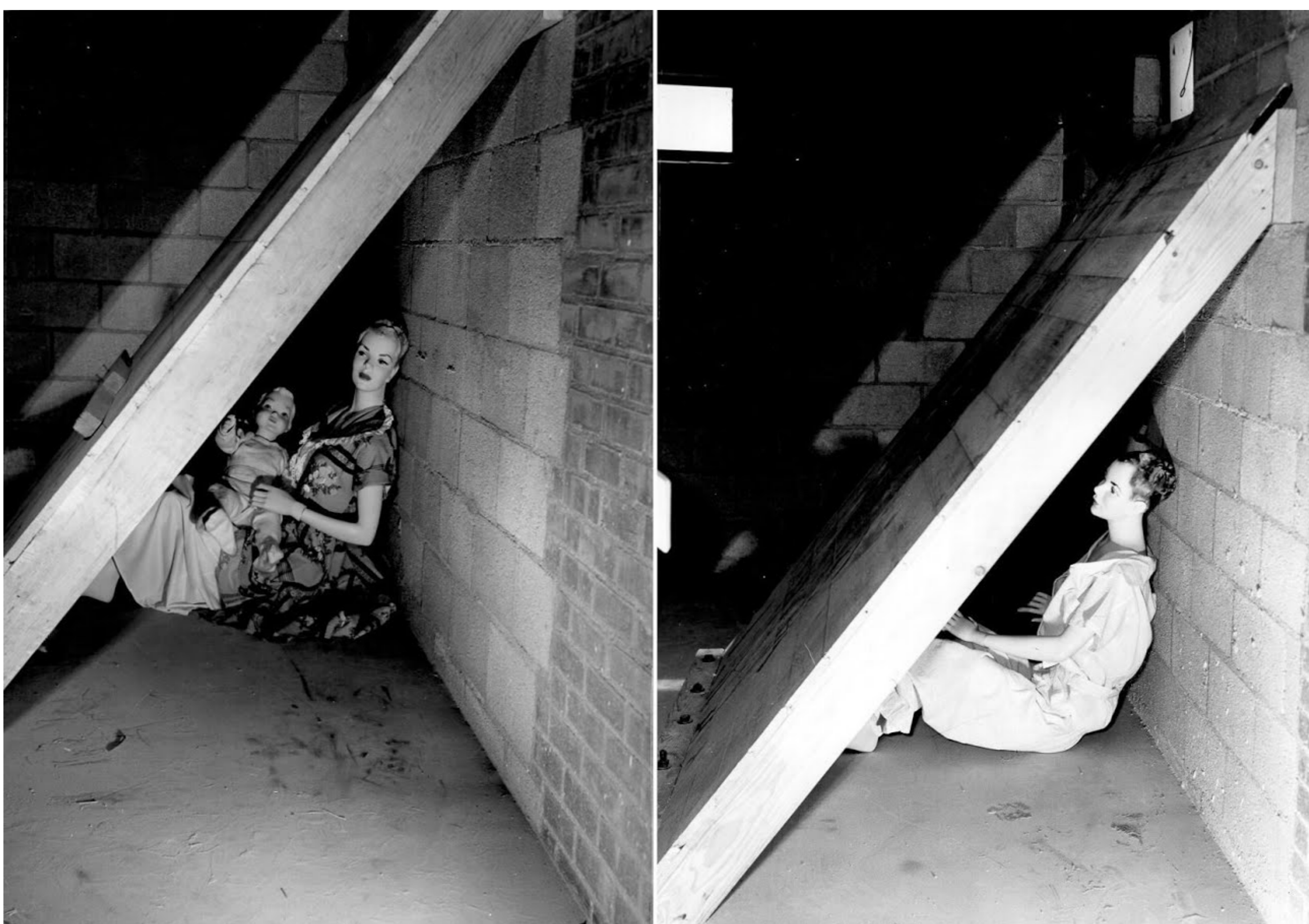
Fig. 16—Lean-to at 7500 ft before blast. Fig. 14—Lean-to at 3500 ft before blast.
